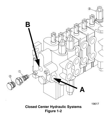
This procedure converts the valve to a closed center operation. If the valve is set for closed center operation, it may be converted back to open center by reversing the above procedure.
